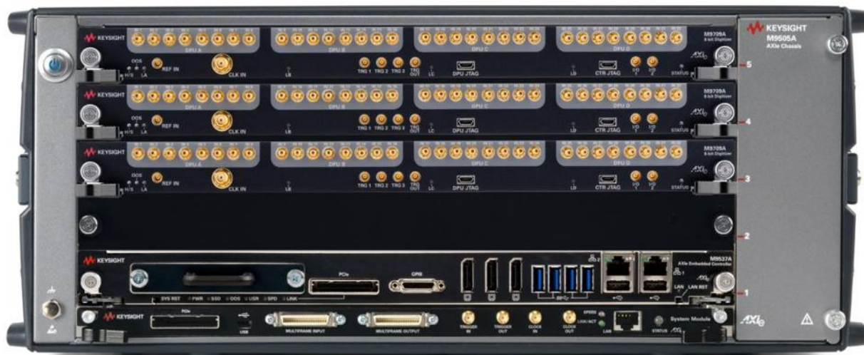
Figure 3. Three M9709A digitizers and an M9537A high performance embedded controller installed in the M9505A 5-slot chassis, forming a 96-ch 8-bit standalone acquisition system.
